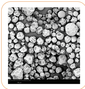
Image of Liposovit® liposome structures using x1000 magnification under scanning electron microscope.
