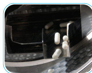
Encapsulation of probiotic powder into 2-piece capsules
