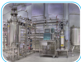
Fermentation tanks culture (grow) probiotic biomass on a large-scale
